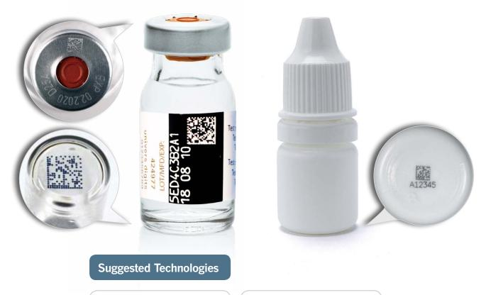
**Continuous Ink Jet** ••• (CIJ) remains an effective marking technology for glass vials. Today's CIJ's use sophisticated software to help ensure high drop placement accuracy, which is especially critical for small 2D codes. Autoclave resistant, visible and UV inks can be used for brite stocking applications.
